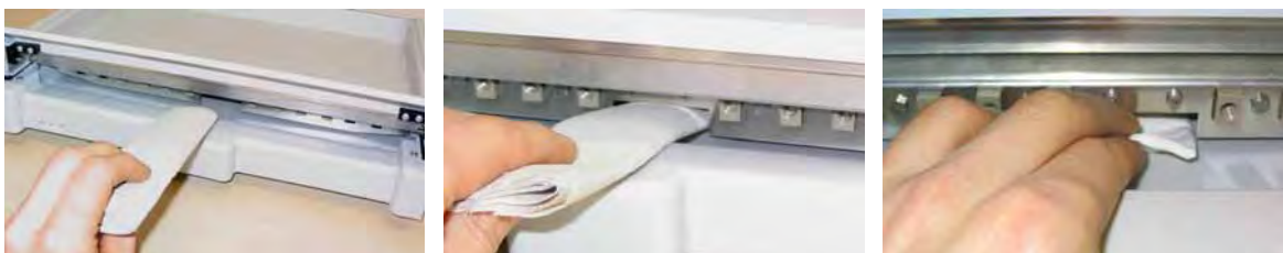
Fig. 10: Drying the leak sensor
